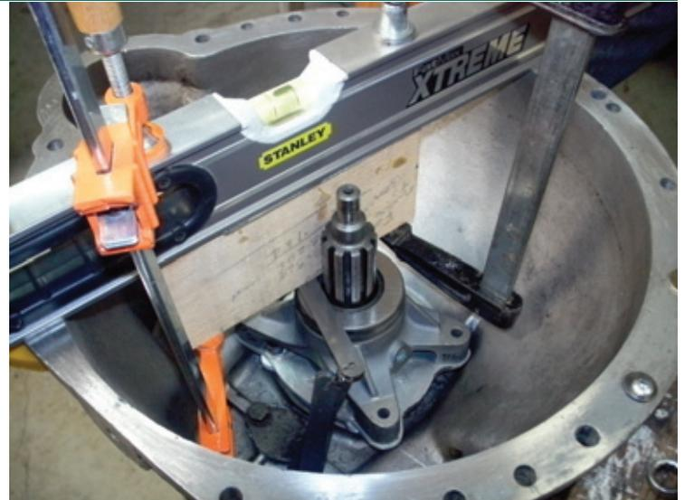
*A hardwood block was used to mimic the intrusion of the clutch fingers into the bell housing - Image: Sean Doherty*
